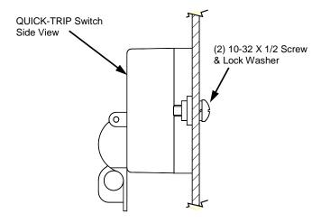
Figure 7.3: QUICK-TRIP Switch Mounting
