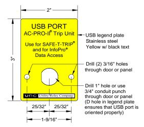
Figure 5.6: USB Extension Plate Drilling
