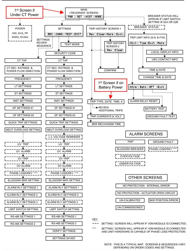
Figure 6.2: Typical AC-PRO-II Menu Navigation Map - Simple View
