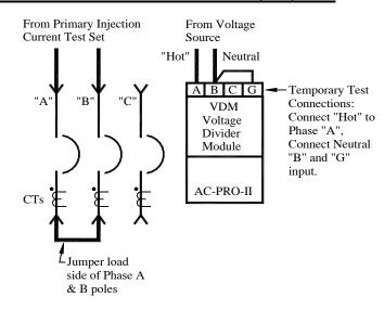
Figure 14.4: Undervoltage Test temporary connections
