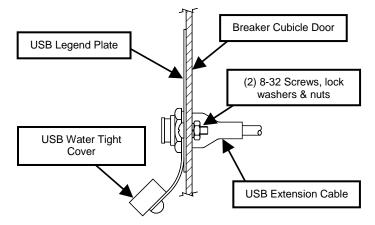
Figure 5.7: USB Extension Plate & Cable Installation
