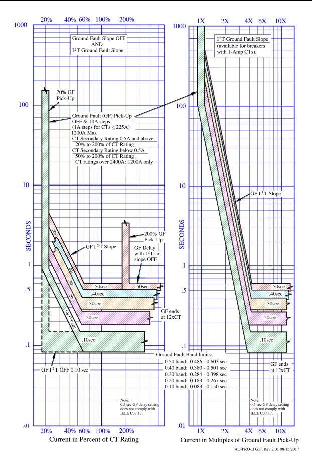
Figure 18.2: Ground Fault (GF) TCC
