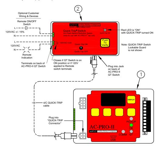
Figure 7.1: QUICK-TRIP System and Connections
