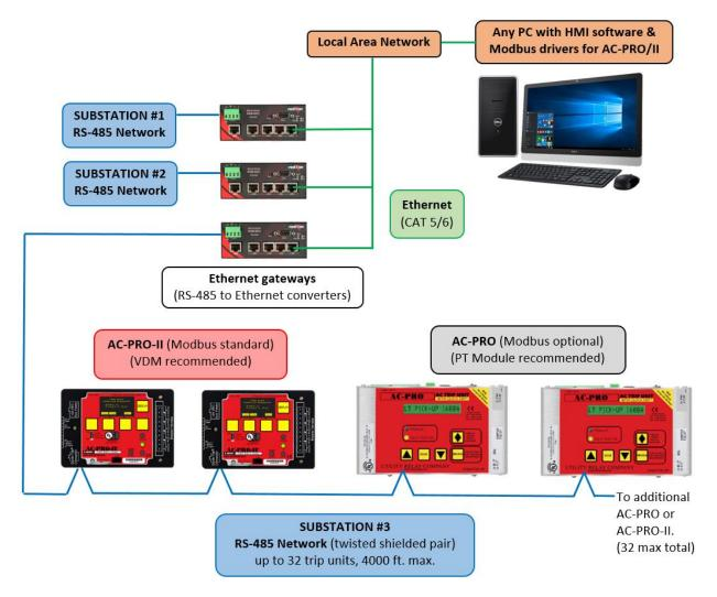
Figure 24.1: Typical Communications Configuration Example
