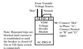
Figure 14.5: Overvoltage Test temporary connections
