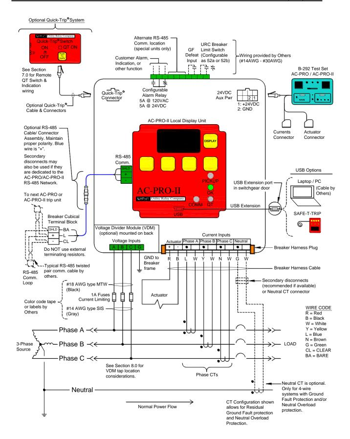
Figure 5.3: AC-PRO-II Typical Wiring Diagram
