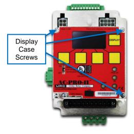
Figure 22.1: Display Case Screw locations
