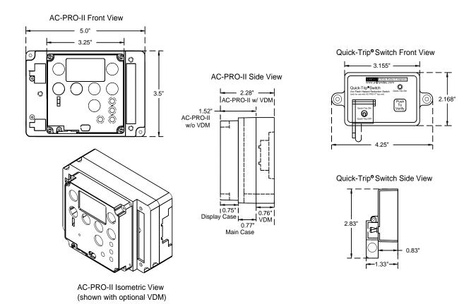
Figure 16.1: AC-PRO-II & Quick Trip Switch Drawings and Dimensions
