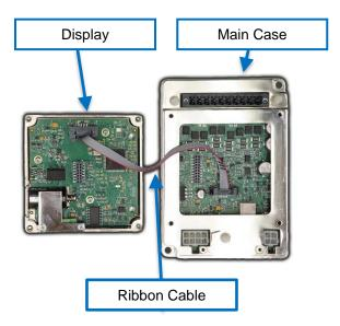
Figure 22.2: Trip Unit and Display (separated)
