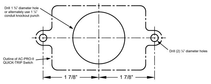
Figure 7.2: AC-PRO-II QUICK-TRIP Switch Drilling Plan
