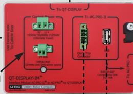
QT-DISPLAY-IM Mounts to back of cubicle door
