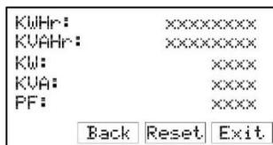
**Figure 13.2: Power and Energy screen (if equipped with VDM)**
