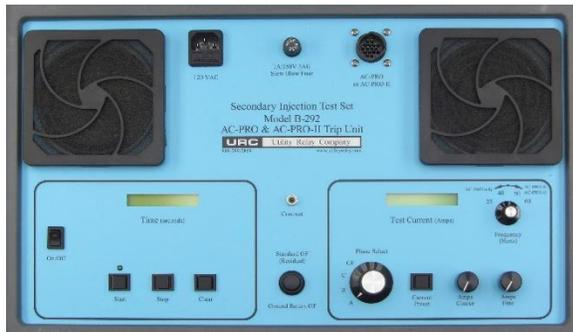
**Figure 15.1: B-292 Secondary Injection Test Set**
