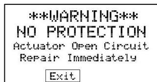
**Figure 20.2: Actuator Open screen**
