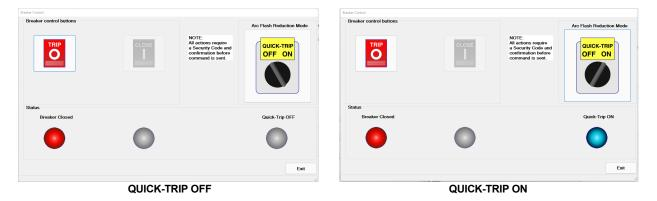
Figure 7.7: Breaker Control Window (InfoPro-AC or Smart 1-Line)
