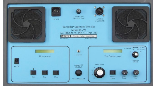
Figure 15.1: B-292 Secondary Injection Test Set
