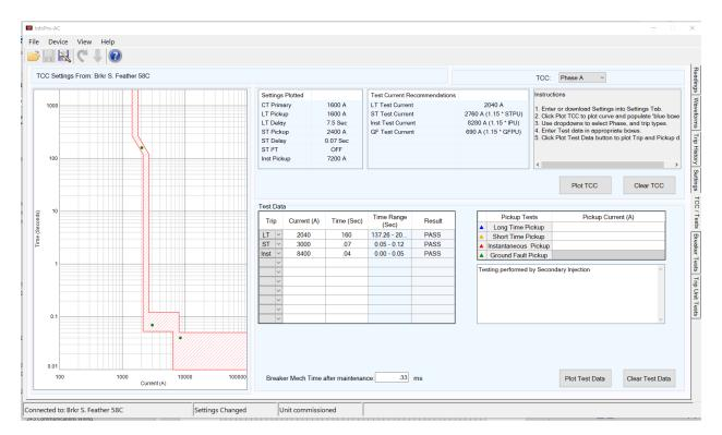
Figure 23.5: InfoPro-AC TCC / Tests Tab
