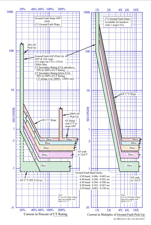
Figure 18.2: Ground Fault (GF) TCC
