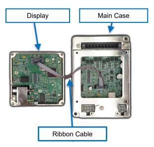
Figure 22.2: Trip Unit and Display (separated)
