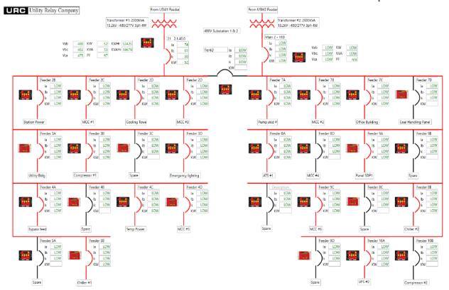
Figure 24.3: Smart 1-Line / Run Mode Example
