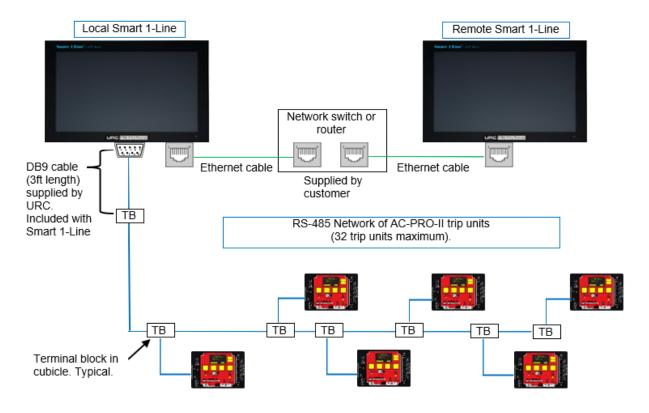
Figure 24.2: Smart 1-Line Communication Solution
