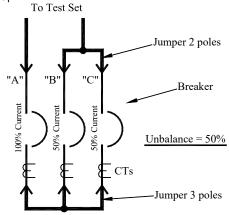
Figure 14.4: Phase Current Unbalance Test
