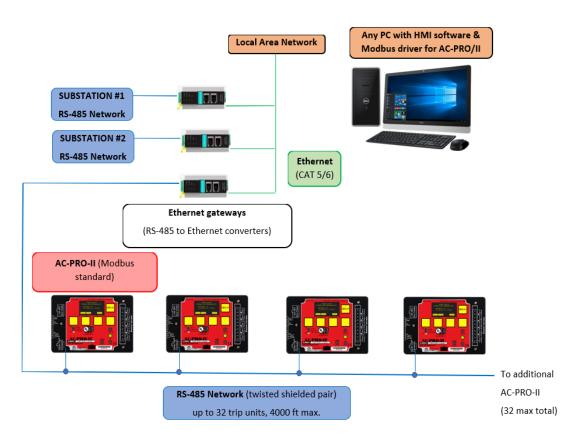
Figure 24.1: Typical Communications Configuration Example
