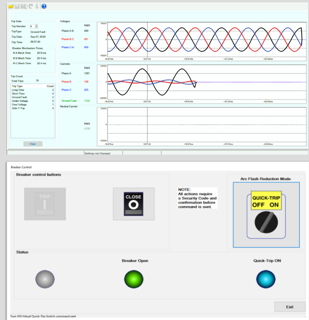
Waveform Capture (top) and the Breaker Control screen (bottom)
