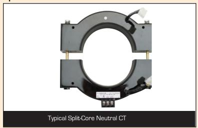
Utility Relay Company manufacturers split core CTs for use as neutral CTs in 4 wire systems. The split cores make it very easy to install the CT on existing bus or cable. Each split core has phenolic plates with punch outs to match standard sizes/shapes of cable or bus-work.
